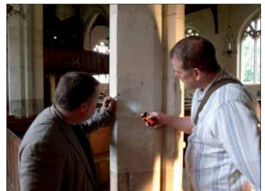
RIGHT: Volunteers using a small LED torch during an initial survey. Small torches and scales fit easily into a coat pocket and can be carried with you during any visit.
